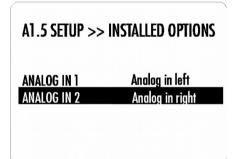
The A1.5 SETUP >> OPTIONS menu provides read-only information about installed slot-in boards. Details are: - ANALOG IN 1: Input board installed in Slot 1
