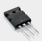
The NA009 is the new power transistor used in the output stage of the Marque Separates power amplifiers. Exclusive for use in Naim amplifiers, the NA009 was over a year in development, with extensive work on the choice of materials, thermal dynamics – the effect of heat on the performance – and die-matching, to ensure consistency between individual transistors.
