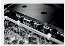
No part of a Naim product escapes the careful scrutiny of our engineers. The position and layout of wires that carry signals and power around a product is very important. Run a delicate audio signal line next to a noisy power line for example, and it will pick up noise and distortion.
