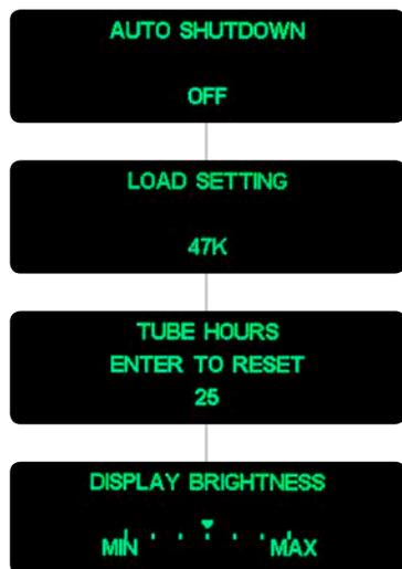
'OPTION' on the front panel or remote to adjust the settings of that particular selection. After making the appropriate change, pressing the 'ENTER' button will confirm the new setting, and the display will show 'OKAY' for five seconds before reverting back to the normal operation screen.
